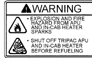
Figure 3: Shut Off Before Fueling Warning
