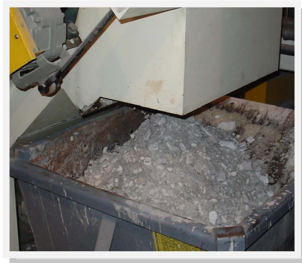
Solid waste being dispensed into a self-dumping hopper.
