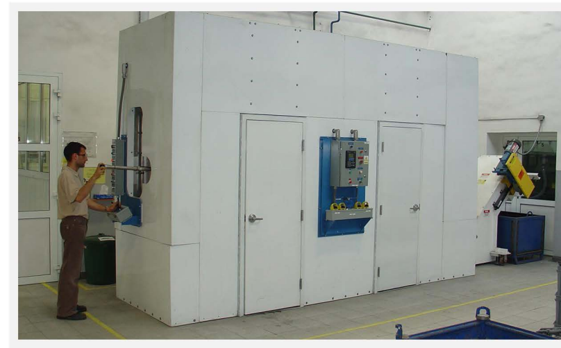
Triplex Systems, Inc. Model TRX-750AM Automatic and Manual Cleaning Centers with common drag conveyor and sound enclosure to meet European CE Sound Standards. Sound enclosures are available as an optional feature.
