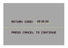
The Return Code for a successful Purge is '20 20 20'. If any code other than '20 20 20' is displayed, contact your service provider for assistance. Press the Cancel key to return to the Diagnostics main menu.
