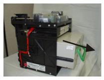
Figure 4-6a. Removing note cassette. (TDM-100)
