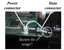
Figure 11. Data / power connections.
