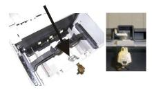
Figure 4-8. Pull the packer plate back. Some cassettes allow the pusher-plate to be latched in position using the key-lock.
