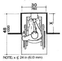
For a front approach, where the depth of the alcove is equal to or less than 24 inches (610 mm), the required clear floor space is 30 inches by 48 inches (760 mm by 1220 mm).
