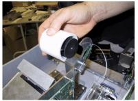
Figure 6-3. Removing paper roll from bracket.
