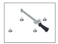
Figure 5. Tighten bolts with tor que wrench.
