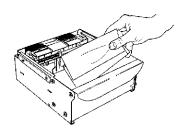
Figure 4-18. Removing rejected notes.
