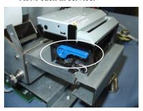
Figure 6-10. Blue tension lever (correct position).
