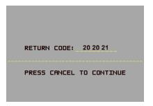
The Return Code for a successful Test Dispense is '20 20 21'. If any code other than '20 20 21' is displayed, contact your service provider for assistance. Press the <u>Cancel</u> key to return to the Diagnostics main menu.
