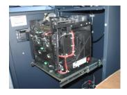
Figure 4-2. Slide dispenser out to fully extended position.
