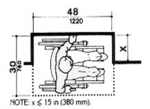
For a side approach, where the depth of the alcove is equal to or less than 15 inches (380 mm), the required clear floor space is 30 inches by 48 inches (760 mm by 1220 mm).
