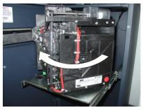
Figure 4-4. Rotate mechanism to service position (clockwise).
