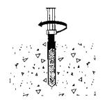
Figure 6. Drive anchor rod into capsule using hammer drill.
