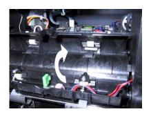
Fig. 7-9. Unlock and lift upper access door to check for stuck notes.
