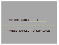
print two lines of 42 characters, fails to advance the paper, or fails to cut the paper, contact your service provider for assistance. A return code of '0' indicates a successful printer test. Press the <u>Cancel</u> key to return to the Diagnostics main menu.
