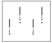
Figure 3. Place anchor bolts in mounting holes.
