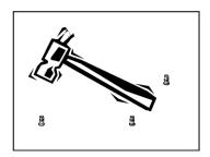
Figure 4. T ap anchor bolts into mounting holes.
