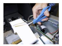
Figure 6-1. Cut paper between the roll and the printer feed path with scissors.
