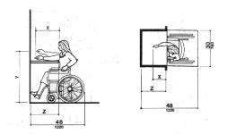
NOTE: x shall be ≤ 25 in (635 mm); z shall be ≥ x. When x < 20 in (510 mm), then y shall be 48 in (1220 mm) maximum. When x is 20 to 25 in (510 to 635 mm), then y shall be 44 in (1120 mm) maximum.
