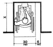
NOTE: If x > 24 in (610 mm), then an additional maneuvering clearance of 6 in (150 mm) shall be provided as shown.
