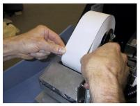
Figure 6-6. Feeding paper into the printer take-up slot.
