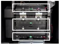
Fig. 7-4. Location of upper, middle and lower access doors.
