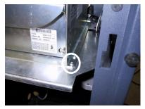
Figure 4. Secure mechanism chassis to tray using two screws.
