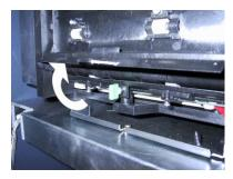
Fig. 7-7. Unlock and lift lower access door to check for stuck notes.
