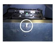
Figure 4-3. Pull release pin for swivel platform.
