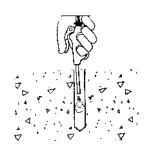
Figure 2. Blow out dust/debris.
