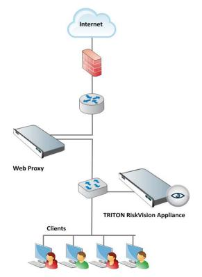
When TRITON RiskVision is positioned downstream from the web proxy, between the clients and the proxy, TRITON RiskVision components see:
