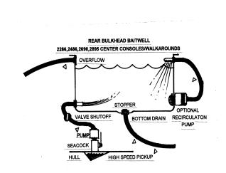
Leaning Post Baitwell: This switch operates a two pump, 50 Gallon, bait well system that is an optional system on most models and popular with serious bait fisherman and tournament anglers alike. There are two1100 GPH pumps that are available for use with this system. Only one pump at a time can be operated on the three way switch located at
