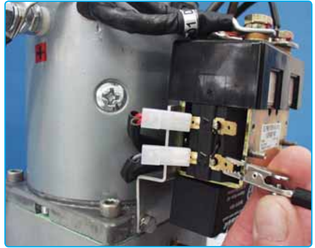
Jumping ground to grey on D1 coil
