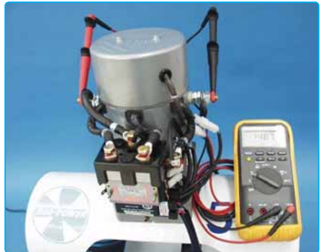
Checking voltage at thruster
