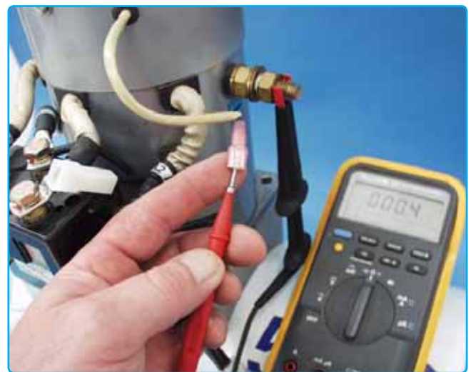
Checking continuity between thermo switch lead and battery negative post
