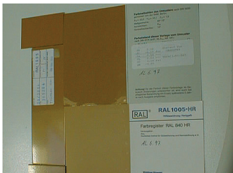
Img. 4.1.1. Color shift between RAL-cards HR and GL
