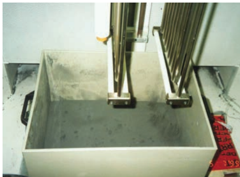
Img. 2.1.1. Fluidization - the powder has to flow like water
