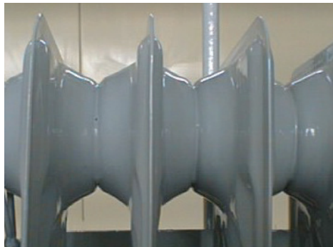
Img. 2.6.2. Rip up caused by poor metal-production
