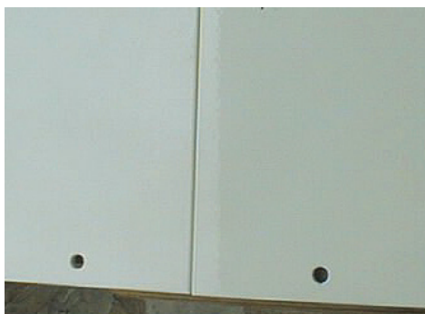
Img. 4.3.1. Different opacity on steel and aluminum
