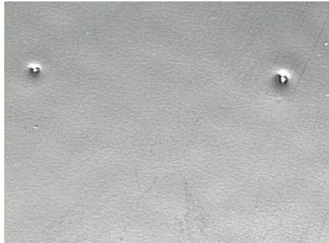
Img. 3.5.5. Bitter pits caused by metal sliver in the underground
