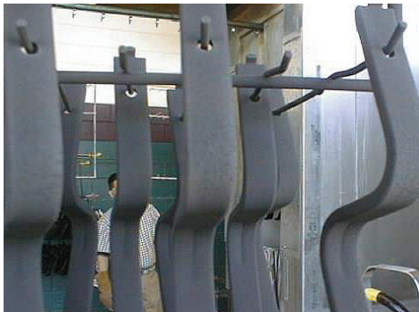
Img. 2.7.1. Film thickness too high (ornateness)
