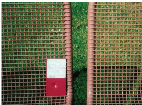
Img. 5.1.1. Chalking caused by faulty powder coating selection
