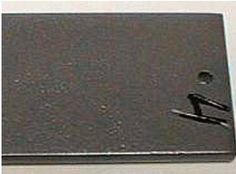
Img. 1.2.4 Crater in powder coating film caused by corrosion
