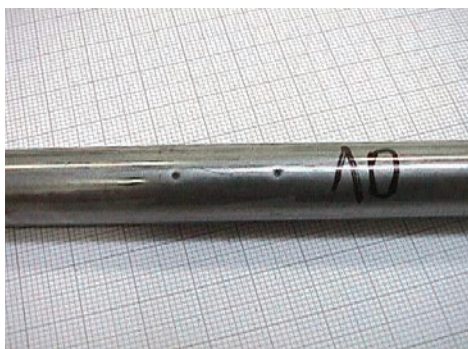
Img. 3.2.1. Crater caused by oil in the compressed air
