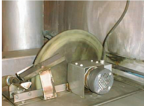
Img. 1.2.2 Primitive alternative of an oil separator
