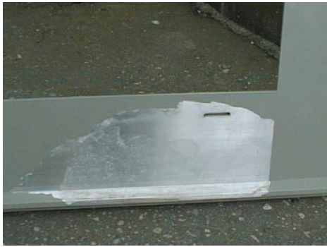
Img. 1.1.2. Poor (no) chromating
