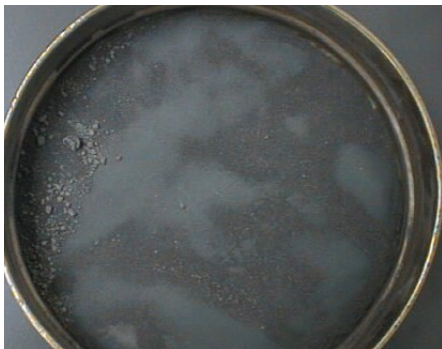
Img. 3.1.1. Filter residues cause powder spitters
