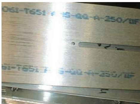
Img. 4.4.1. Stamping ink (untreated)
