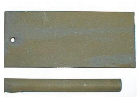
Img. 1.2.3 Corrosion caused by Fe-phosphating on radiated pieces
