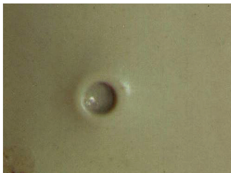
Img. 3.6.5. Bubbles caused by tassels in the galvanized plate
