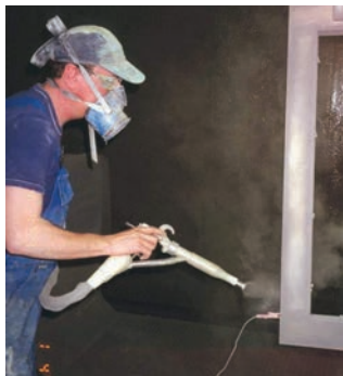
Img. 2.6.1. Additional earthing for hollows
