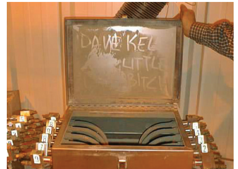
Img. 2.1.2. Poor fluidization - too much powder
