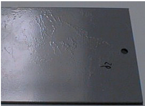
Img. 1.2.7 Poor purging, radiated, KTL-grounded
