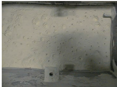
Img. 2.1.2. Poor fluidization
