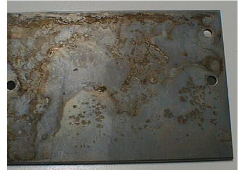
Img. 1.2.6 Poor purging, afterwards stored wet
