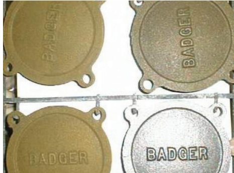
Img. 1.2.5 Corrosion of sandblasted work pieces after pretreatment
