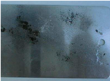
Img. 1.2.1 Fat-arrears after pretreatment
