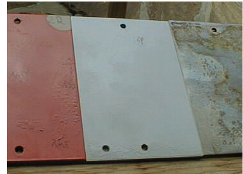
Img. 1.2.9 Poor purging, radiated, KTL-grounded and powder coated - comparison
