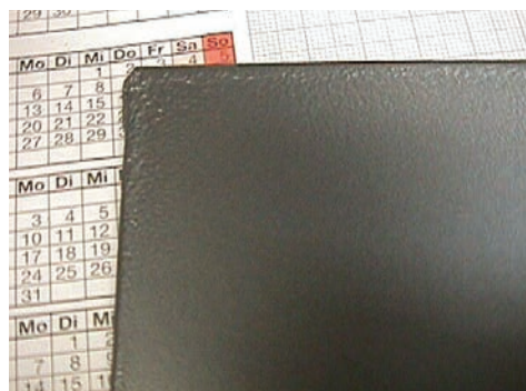
Img. 3.4.1. Boil up of the coating caused by a too high film thickness
