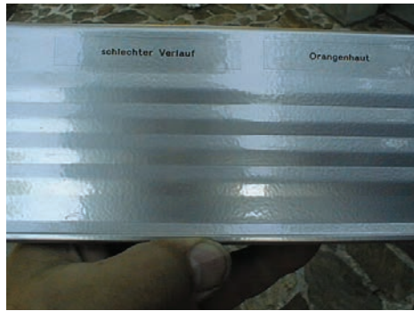
Img. 3.8.2. Orange peel effect
