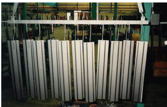
Img. 2.g.1. Unsteady film thickness because of wrong mounting (to narrow distances)
