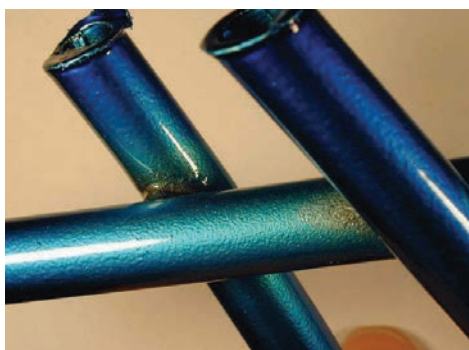
Img. 7.3.1. False position caused by incompatibility of the flux
