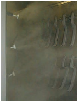
Img. 2.7.2. Too thick powder cloud
