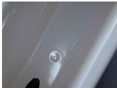
Img. 3.2.2. Crater caused by oil residue
