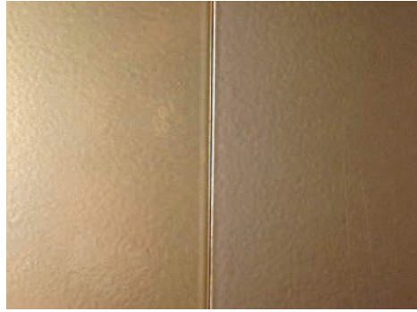
Img. 7.3.5. Color-deviation at dormant caused by two different shades in the oven
