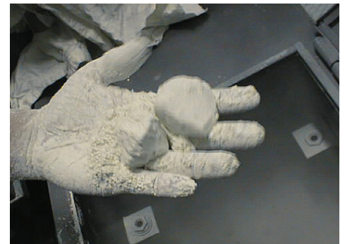
Img. 2.5.1. Powder lumping in the box
