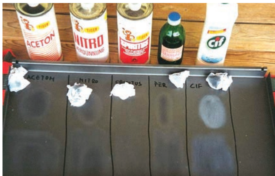
Img. 7.2.1. Greying caused by cleaning compounds
