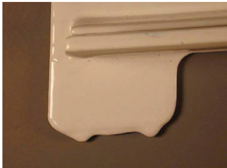
Img. 3.7.1. Drop formation caused by a too high film thickness
