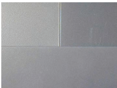
Img. 7.3.2. Color variations caused by reclaim
