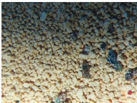
Img. 6.1.5. Dust in the reclaim powder (enlarged)
