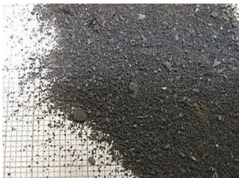
Img. 6.1.4. Dust in the filter residue
