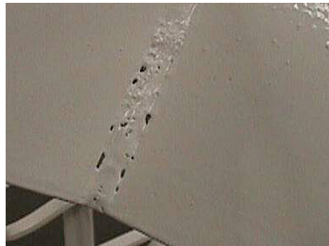
Img. 3.9.2. Insufficient wet out caused by oilcoat
