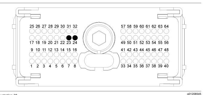
Typical view of the P1 pin locations for the diagnostic and Perkins Data Link connectors (24) Perkins Data link (PDL) -
