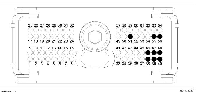
Typical example of the P2 pressure sensor pin locations
