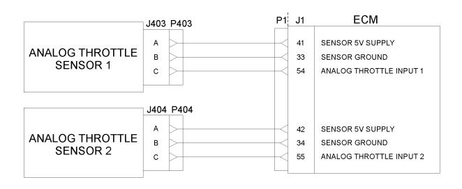
Typical example of the schematic for the P1 OEM connections for the analog throttle demand sensors
