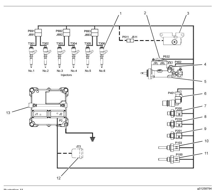
Schematic diagram for the 1106D engine
