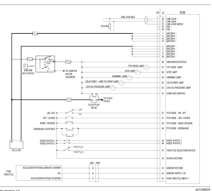
Schematic Diagram for a Typical Application
