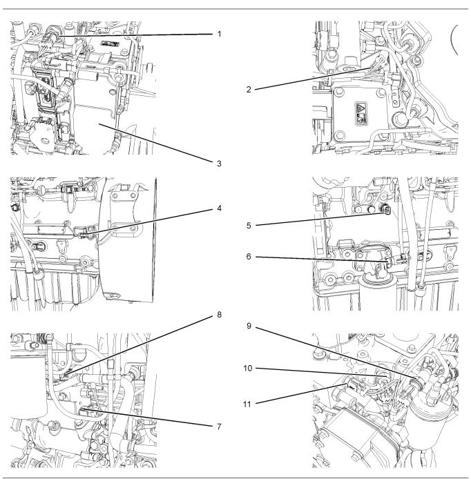
Illustration 7 Close up views of the sensor locations on the 1104D engine
