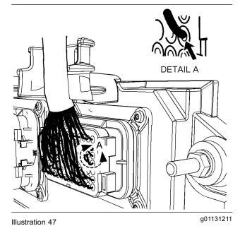
Leaky seal at the connector (typical example)
