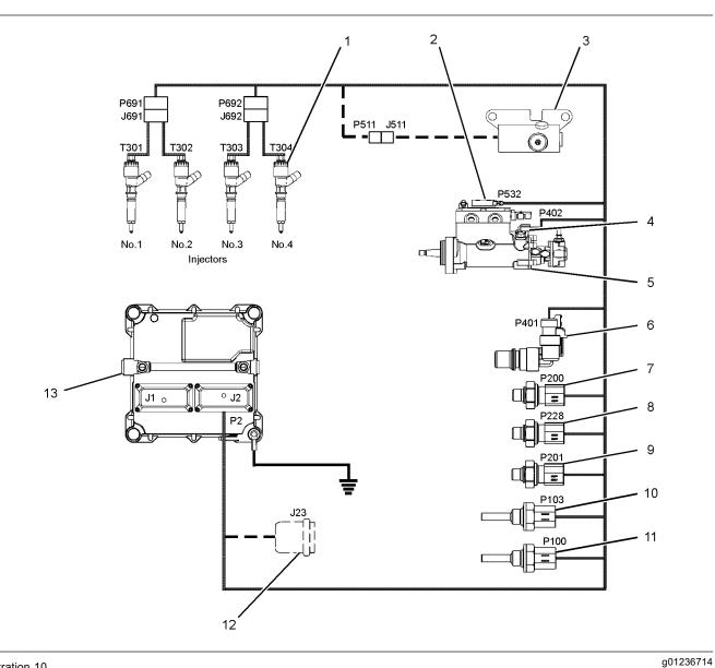
Schematic diagram for the 1104D engine
