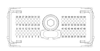
Illustration 15 Layout of the Connector Pins (view from the rear)
