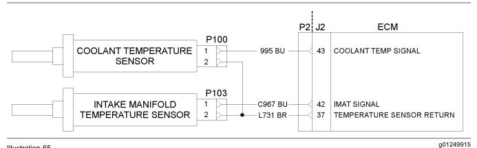
Schematic for engine temperature sensors
