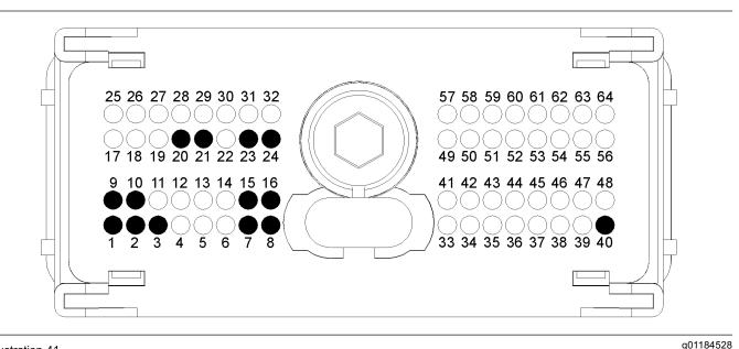
Typical view of the P1 OEM connector pin locations for the diagnostic and Perkins data link connectors
