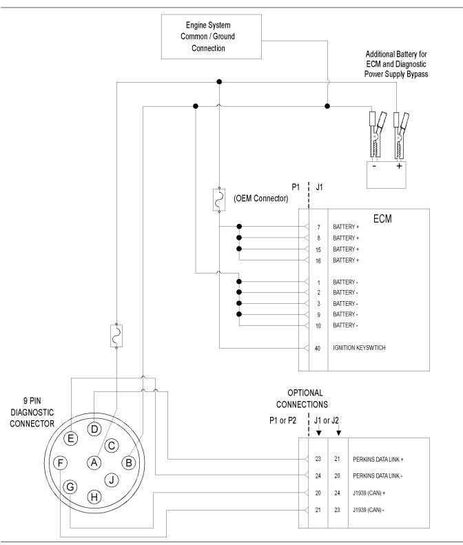
Schematic of the bypass harness connector
