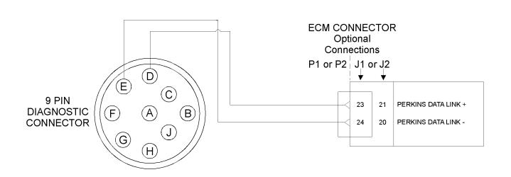
Schematic of the diagnostic connector and the Perkins Data Link connector
