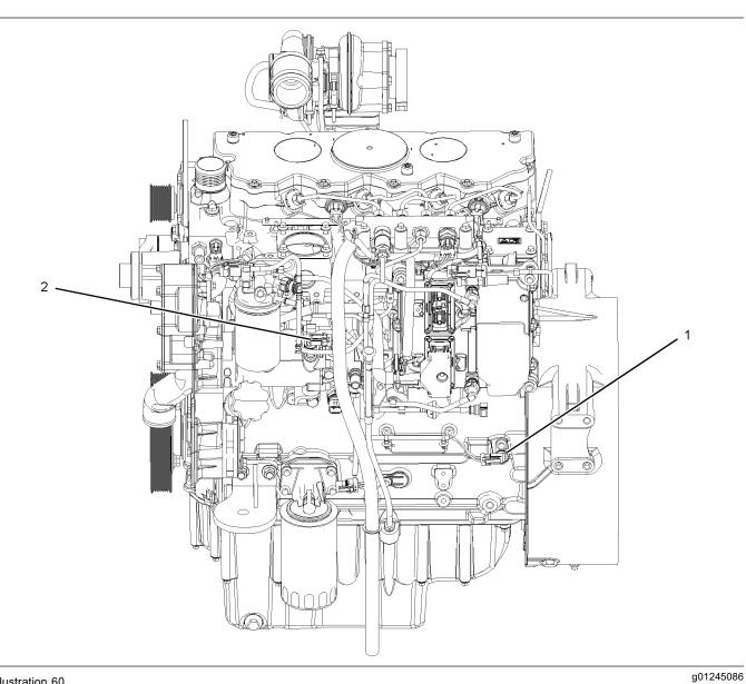
Typical view of the locations for the speed/timing sensor on the 1104D engine
