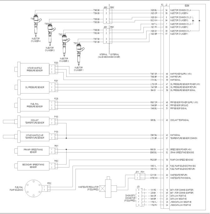
Illustration 12 Schematic Diagram for the 1104D Engine Harness
