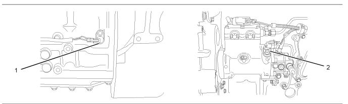
Detailed view of the sensor locations on the 1106D engine
