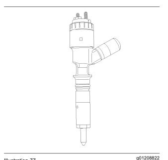
Illustration 77 Typical example of the electronic unit injector
