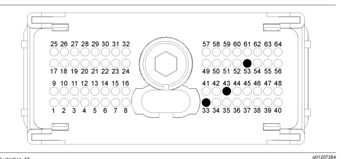
Typical example of the pin locations on the P1 connector
