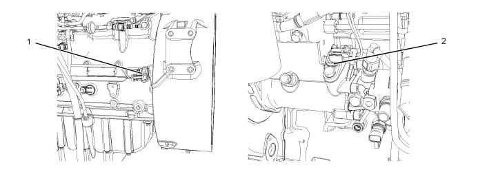
Detailed view of the sensor locations on the 1104D engine
