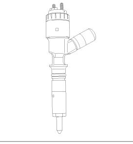
Illustration 78 Typical example of the fuel injector
