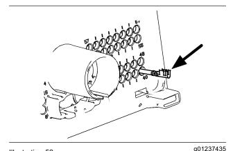
Illustration 52 Diagram for testing pin retention
