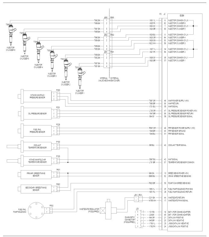
Schematic Diagram for the 1106D Engine Harness
