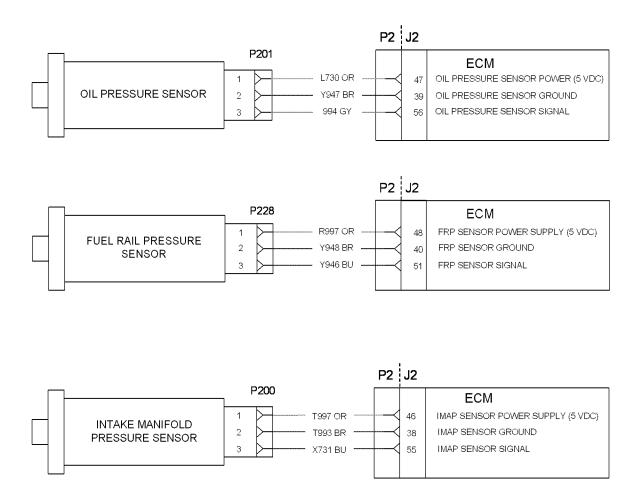
Typical example of the schematic for the sensors
