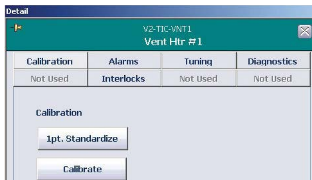
Figure 2.41. Vent heater detail screen.
