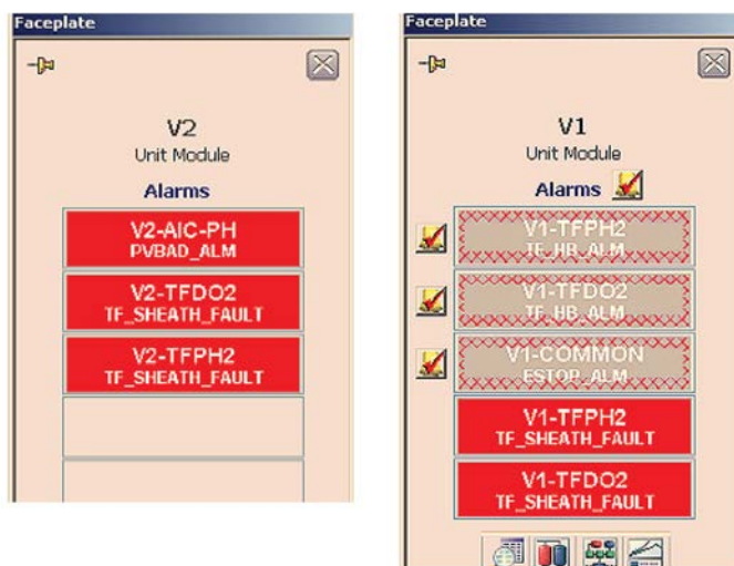
Figure 3.14. Active alarm showing flashing boxes (left) and acknowledgement box (right).
