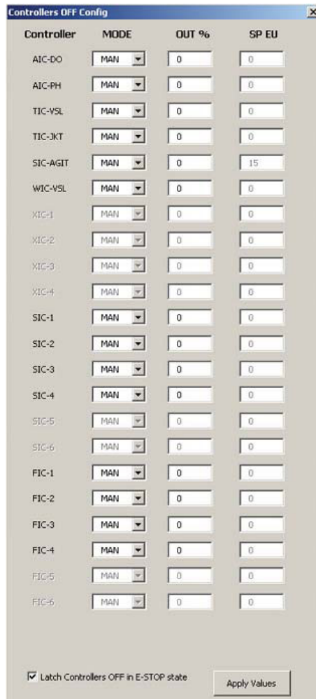
Figure E.1. Controllers Off config screen.
