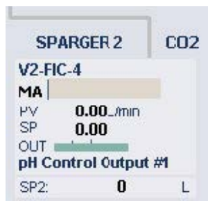
Figure 1.12. Control box Sparger 2 detail on main screen.
