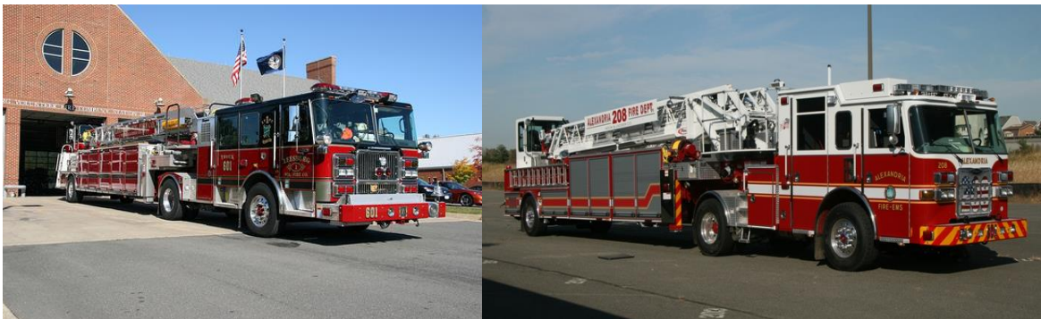
Figure 4: Tractor-drawn aerial devices, or tiller trucks, are referred to as truck companies.
