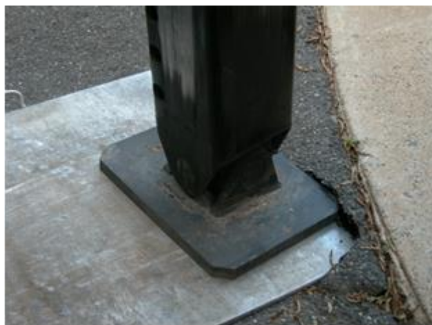
Figure 20: Jack plates should be centered over the outriggers.
