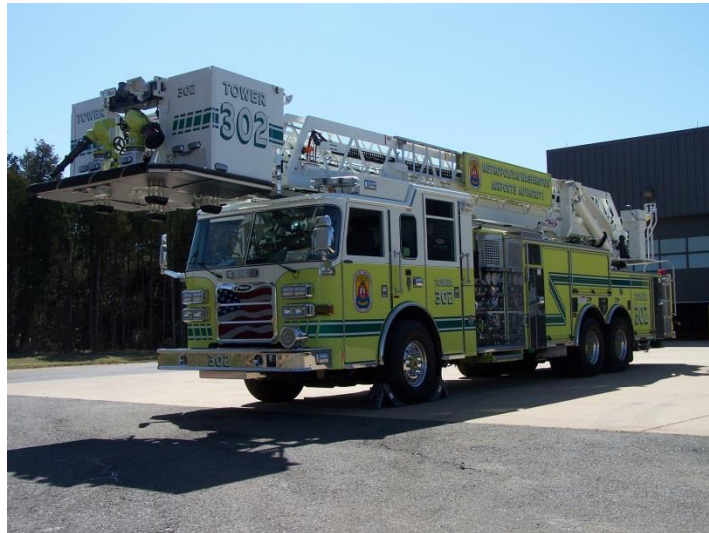
Figure 5: A quint provides the features of both an engine and a tower.
