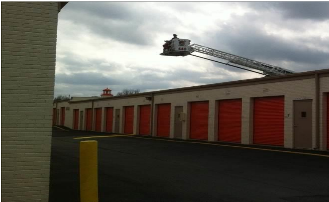
Figure 29: Truck companies should use the reach of the hydraulic ladder during advanced fires by positioning on a parallel alley and projecting the master stream over and into the involved unit(s).
