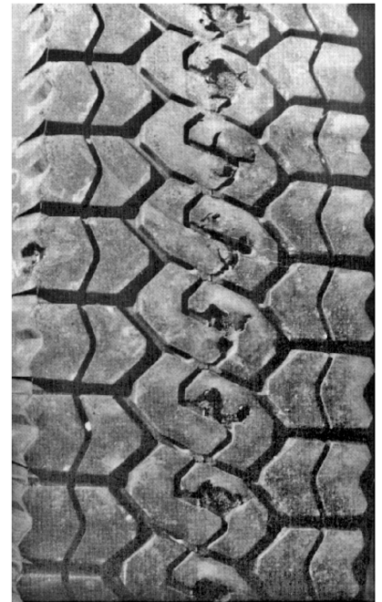
Example of Dyno Damage
