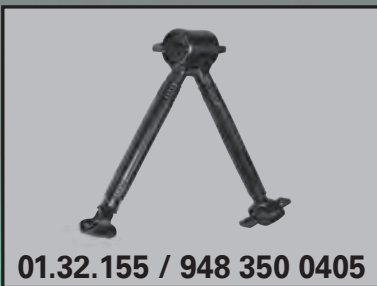
Track control arm Rear axle, triangular arm Length: 622 mm OD: 56 mm
