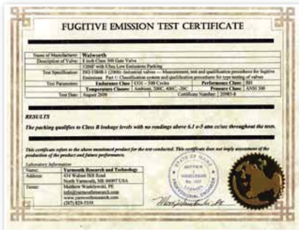
Emissions after 500 cycles at ambient and 350 °F issued by Yarmouth Research and Technology Lab for 8 inch Class 300 Gate Valve After 500 cycles the measurement result was less than 50 ppm.
