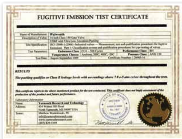
Emissions after 500 cycles at ambient and 350 °F issued by Yarmouth Research and Technology Lab for 16 inch Class 150 Gate Valve After 500 cycles the measurement result was less than 50 ppm.
