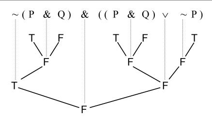
In the above diagrams, the broken lines indicate, in each simple computation, which truth function (connective) is employed, and the solid lines indicate the input values.
