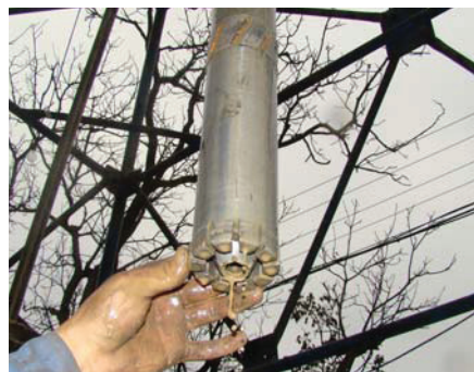
Figure. 6 the core claw gathering up photo in the ground
