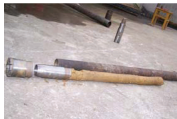
Figure. 5 the core photo in the soft stratum
