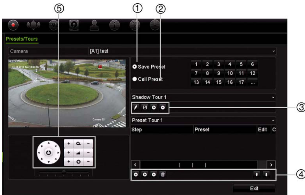
Figure 23: PTZ configuration window
