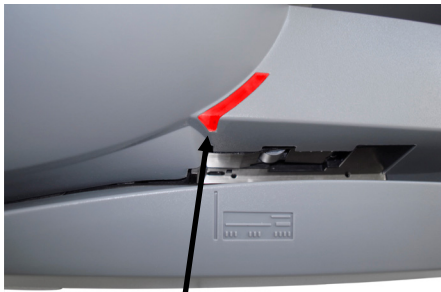
Fig. 9: The LED comes on 'Red' to indicate power to the unit.
