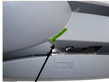
Fig. 10: When the scanner is acquired by the application, the LED turns green.
