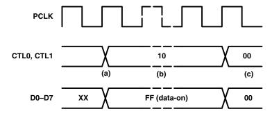
Figure 26. Null Packet Reception Timing
