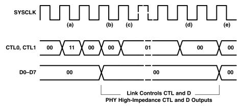
Figure 16. Cancelled/Null Packet Transmission
