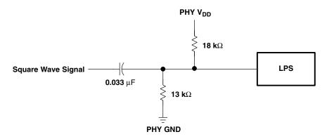
Figure 8. Isolated Circuit Connection for LPS
