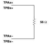
Figure 1. Test Load Diagram
