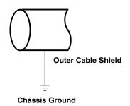
Figure 6. Non-DC Isolated Outer Shield Termination
