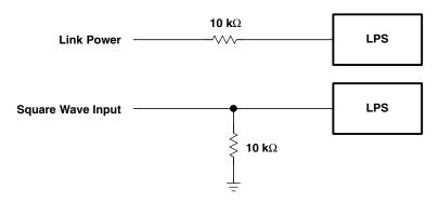
Figure 7. Nonisolated Connection Variations for LPS
