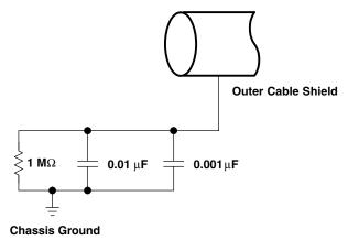
Figure 5. Typical DC Isolated Outer Shield Termination
