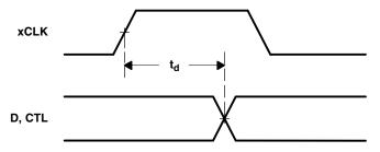
Figure 3. Dx and CTLx Output Delay Relative to xCLK Waveforms
