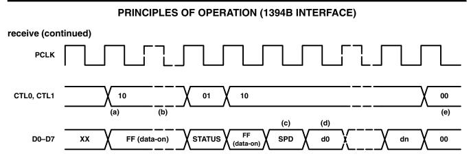
NOTE A: SPD = Speed code, see Table 35. d0-dn = Packet data. STATUS = status bits, see Table 32.
