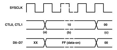
Figure 14. Null Packet Reception Timing
