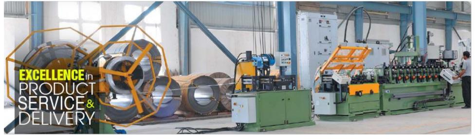
We have a sophisticated 'U bending facility' to cold bend tubes of 15.87mmOD to 25.4mmOD and up to 3.05 mmwall thickness with 25.4mmto 1000mm Center line radius and with leg length up to 14meters.
