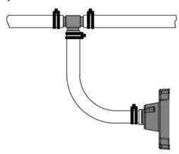
For aircraft with ¼ inch static lines, two adapters are provided which can convert from ¼ inch inside diameter hoses to the 5 mm hose in the install kit.
