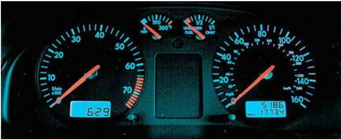
Fig. 3.5. Automotive dashboard back-lit with blue LEDs.
