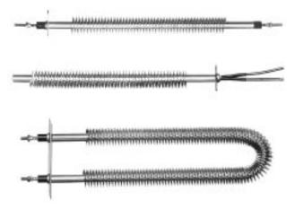
**Standard Construction:** A corrugated 304 stainless steel fin is helically wound on a .475" diameter 304 stainless steel element. To insure a permanent bond, each end of the fin is tack-welded to the element sheath. The entire assembly then goes through a computer controlled atmosphere furnace. This process prepares the element to be bent into a variety of configurations. Standard fin density is five fins per inch, while eight fins per inch can be furnished when specified.
