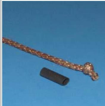
Heat shrink tubing can protect the line from the sharp inside edge of the hole.
