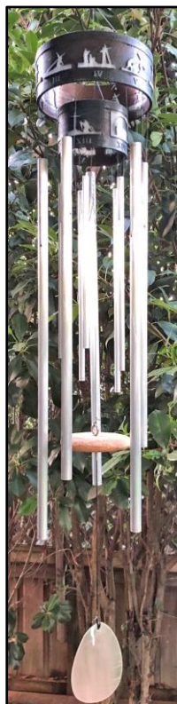
Gift for a special mother-in-law by Gary Kester. Top support was 3D modeled and printed in PLA+ plastic for this 10-chime
