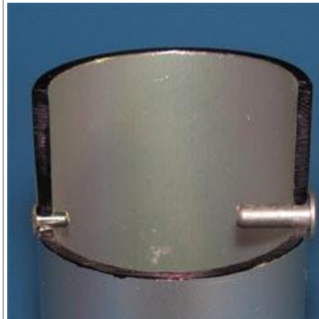
1/8 inch and 3/16 inch eyelets using the shell from a pop rivet. Use only for thru line.
