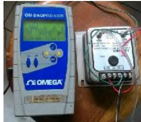
Gambar 3.20 DAQ data logger dan Differential pressure transmitter
