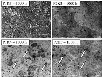
Figure 9: SEM micrographs (x500) of HVOF and HVAF coatings exposed to cyclic corrosion test after 1000 hours
