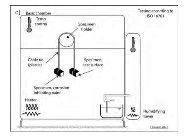
Figure 1: Wear resistance tests: a) ASTM D6037, b) ASTM G65 and c) cyclic corrosion test according to ISO 16701.
