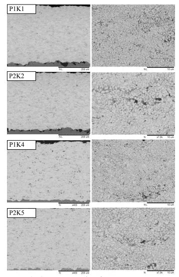
Figure 2: SEM micrographs of respective coating cross sections (X400- left; X7000-right)
