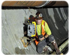
Project Surveyor Sean Fitzpatrick, PLS, operates a Trimble S6 in the Bay Tunnel. Remote control and automated pointing enables him to quickly capture precise measurements to tunnel control points.
