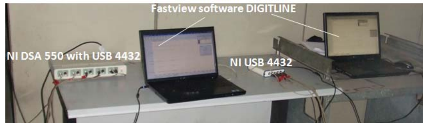
Fig.3. The experimental setup for control room measurement data
