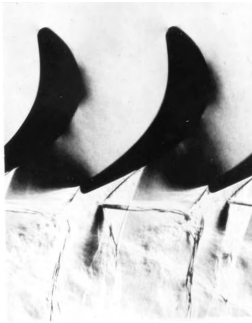
Figure 16. Exit shock system for an axial turbine cascade M = 1.33 .
