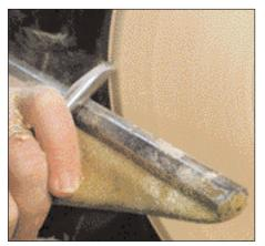
With a <sup>3</sup>/8" bowl gouge, keep the handle perpendicular to the surface. The tool rest is positioned at 45 degrees.
