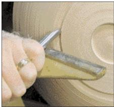
Use the tip of your bowl gouge to define the perimeter of the platter's foot. This photo shows detailing a chamfered foot.
