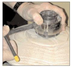
Lightly tighten the scroll-chuck jaws in the recess. To check for proper seating, rotate the chuck before fully tightening.
