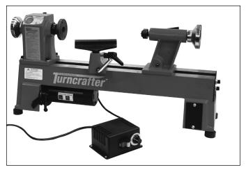
▲ The control box for the **TCLPROVS** can also be easily mounted anywhere that is convenient for you. The 3' cord from the motor to the control box allows you that flexibility.
