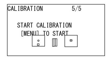
This screen allows you to calibrate the analog channels (A1..A7).
