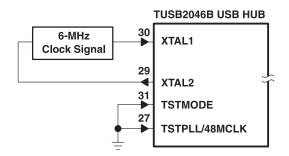
Figure 5. 6-MHz Input Clock Configuration
