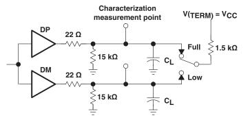
Figure 1. Differential Driver Switching Load
