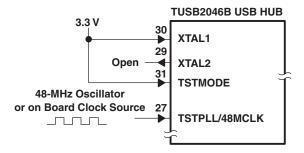
Figure 7. 48-MHz Input Clock Configuration
