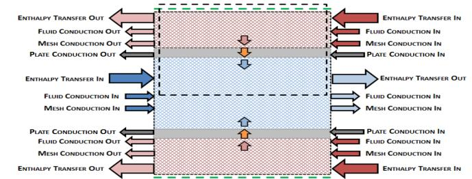
Axial conduction losses – which may be significant in high-ε designs – are captured for both the parent material and the heat transfer enhancing structures
