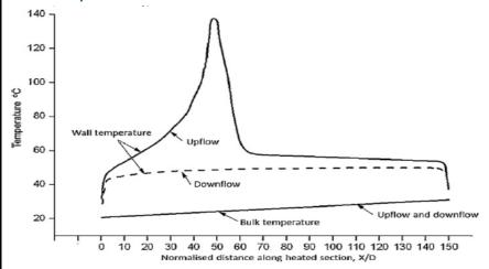
Fig. 10. Further reduction of flow rate, 5 mm diameter tube, upflow and downflow. Pressure 7.58 MPa; mass flow rate 0.0129 kg/s; wall heat flux 68 kW/m<sup>2</sup>; Re  $\sim4\times10^4$ .
