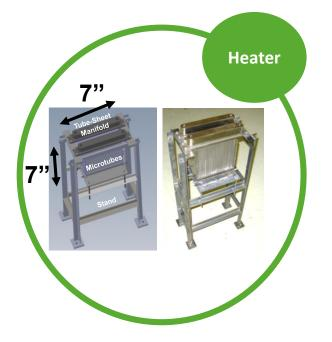
Microtube Cross-flow, Counter-current Heater
