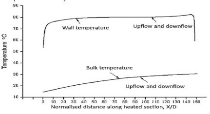
Fig. 9. Highest mass flow rate, 5mm diameter tube, pressure 7.58 MPar, upflow only. Mass flow rate 0.0645 kg/s; wall heat flux  $455 \text{ kW/m}^2$ .
