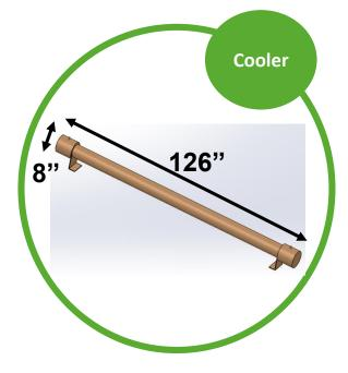
Counter-flow, Shell & Tube Water Cooler
