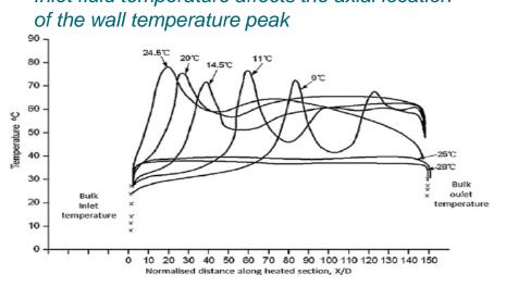
Fig. 8. Effect of reducing inlet fluid temperature, 8 mm diameter tube, upflow only. Pressure 7.58 MPa; inlet temperatures, 9 °C, 11 °C, 14.5 °C, 20 °C, 24.5 °C; mass flowrate 0.02 kg/s; wall heat flux 33.6 kW/m<sup>2</sup>; Re  $\sim$  4  $\times$  10<sup>4</sup>.
