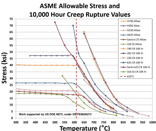
**Design T** increases material strength drops & corrosion rates increase
