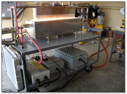
Radiant (High Flux) Test Rig
