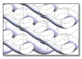
Wire-mesh analysis for creep and pressure-fatigue simulation.
