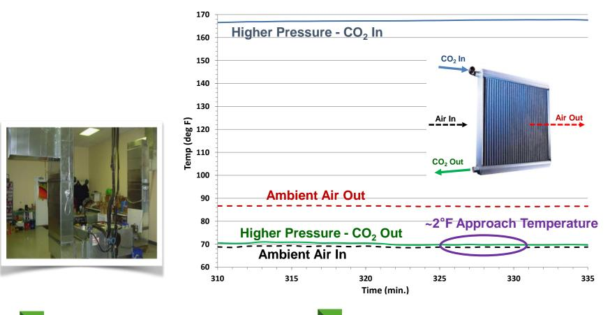
At Thar's test facility, air and CO<sub>2</sub> approaching temperature as low as 2°F was achieved using micro-channel coil.
