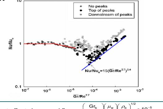
The onset of buoyant effects in upward flow:
