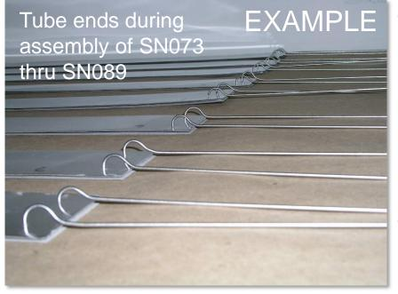
This final batch of heat exchanger cells were of high quality, leak tight and suitable for creep tests
