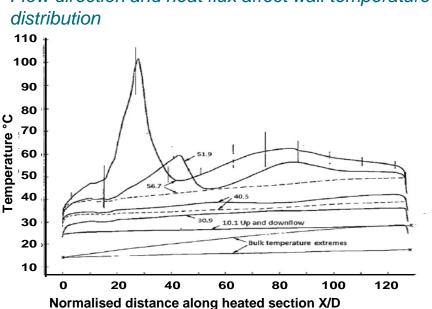
Fig. 4. Localized deterioration of heat transfer with upward flow; 19 mm diameter tube. Upflow is denoted by solid lines; downflow by broken lines, mass flow rate 0.160 kg/s; bulk inlet temperature  $14 \,^{\circ}$ C; wall heat flux as indicated, 30.9, 40.5, 51.9, 56.7 kW/m<sup>2</sup>.
