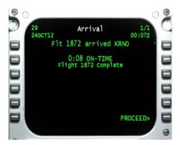
We can see that we arrived 8 minutes early, which is well within our on-time arrival window for this flight. Since this is a passenger flight, we will turn off the seat belt sign and press the LSK6R (PROCEED) key to start the unloading process. This will result in advancing us to the Flight Complete page:
