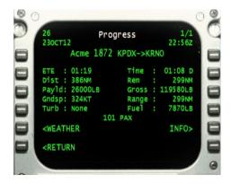
There are two important pairs numbers to compare against one another. The first pair is the "Block ETE" value versus the "Estimated Time Remaining" value for the flight.
