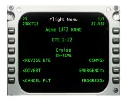
This screen is accessed normally by pressing the **INIT / RST** key on the FCDU's keypad. The Flight Menu gives you a good overview of general items (time, flight number, ETE, and whether you're on-time or not) along with the phase of flight that you're currently in.
