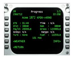
In addition to the Zulu Date and Time, we are reminded that this is flight 1872 to KRNO, the current Distance remaining to our destination, our onboard Fuel, the relative degree of turbulence that our passengers are experiencing, and the remaining ETE in block time. The *ETE* value will be green for normal en-route flight time, will switch to white when we are within our arrival time window, and will turn red if we are officially late.
