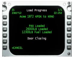
After 15 minutes (which can vary from flight to flight), we can see that all three rows are noted as *Loaded* and the cautionary message *Auto-Load in Progress* has changed to *Door Closing*.
