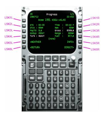
Line Select Keys are referred to in a unique way. The 6 keys on the left-hand side of the control unit are named LSK1L (LINE SELECT KEY 1 LEFT- the key on top) LSK2L (the key immediately beneath LSK1L) through LSK6L (the key on bottom). Unsurprisingly, the 6 keys on the right-hand side are named LSK1R (LINE SELECT KEY 1 RIGHT) through LSK6R.
