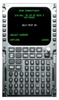
If this screen does not appear on power-up of the device, an error message screen will appear instead, indicating that the Communicator system devices are not configured properly, or are malfunctioning.
