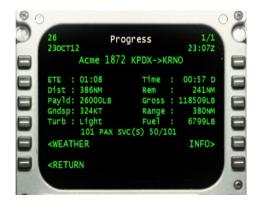
Other important data items are: Gross Weight (*Gross*) which is the weight of the airplane, cargo, passengers, and fuel, and will be highlighted in white if it's greater than the maximum landing weight. (Doing so won't necessarily damage your aircraft, but it will have to undergo strict maintenance protocols after you turn over the keys. Doing so very often won't make Operations happy.)
