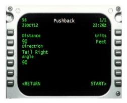
By default the pushback is set to 90 feet back (or less if your airplane is a small one) and then a 90 degree turn with our tail towards the right. You can adjust this by using the appropriate Line Select Keys. In our case 90 feet is good enough, but we need to have our tail turn to the left. So we press **LSK3L** until the option *Tail Left* appears. The result is:
