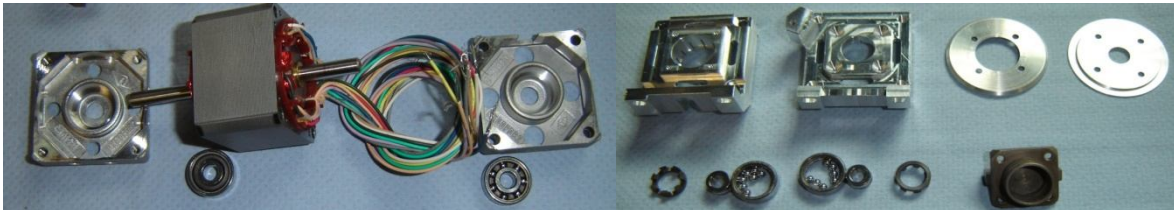
Figure 6: Regular stepper motor preparation for cryogenic operation: Casted parts are replaced by polished metallic surfaces to prevent outgassing and the bearings are replaced for special dry cryogenic bearings. Cryogenic components are on the right.
