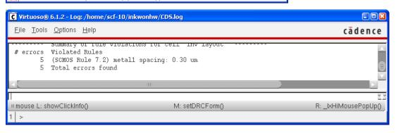
We have five errors. It is because a gnd metal layer is too close to an nmos transistor. After modifying layout, run DRC again.
