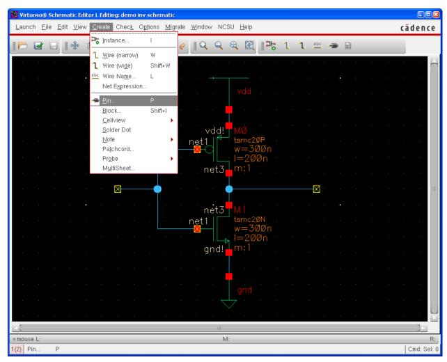
We have for different types of direction. For schematics, we only use two types, input and output. InputOutput type is for supply changes, and it is necessary only for layout. We will discuss about this later.
