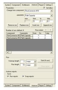
For this example, the 'FlowConnector #10' has been selected and the 'Path:Capacity' parameter. The values shown in the row below are the current value, and the values it will hold once the simulation is running. The user is able to change the 'From', 'To' and 'Step' values as she sees fit. In the picture, the values have a step of .1, and changes from 1 to 1.1.
