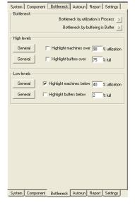
The Bottleneck section already has identified the component named 'Process' to be the utilization bottleneck, and it can be identified by clicking on the '>' button. Red lines appear surrounding the component. The buffering bottleneck has been identified as 'Buffer', and can identified in the same way as previously mentioned.
