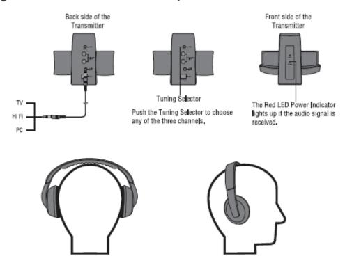
Switch On the headphones. Push the Tuning Selector to obtain the proper channel. The red LED will keep flashing during the selection. When the proper channel is obtained, the red LED will stop flashing.
