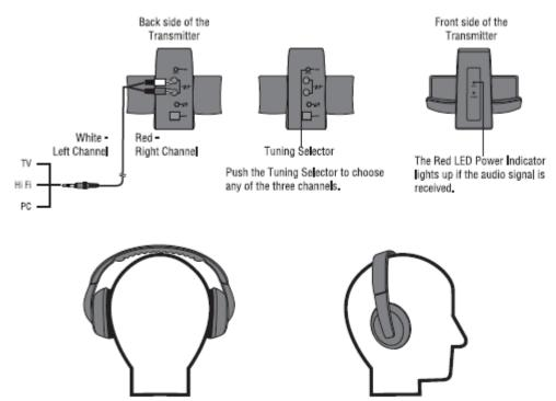
Switch On the headphones. Push the Tuning Selector to obtain the proper channel. The red LED will keep flashing during the selection. When the proper channel is obtained, the red LED will stop flashing.
