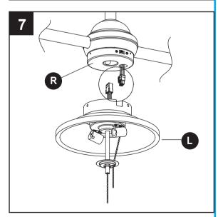
8. Align the cutout on the light kit (L) with the reverse switch on the bottom housing (R). Attach the light kit (L) to the motor housing (G) using the three set screws previously removed (step 6, page 12). Tighten securely, then install bulbs (M) into each socket.
