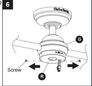
To install the light kit (L), attach the connector preassembled on light kit (L) to the connector preassembled on bottom housing (R).
