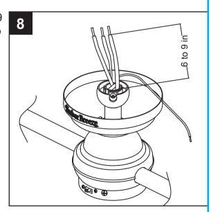
Carefully lift the assembly and rest the hanger ball of downrod assembly (B) on the mounting bracket (A) attached to the outlet box.
