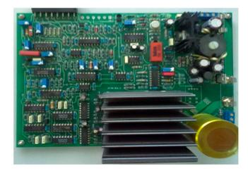
Figure 4. DC motor driver (60 V, ±10 A) [21].
