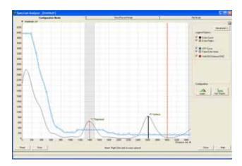
With Rosemount RadarMaster, a noise threshold curve and false echo registration can automatically be created by clicking the Learn button.
