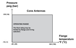
Process temperature and pressure diagram.
