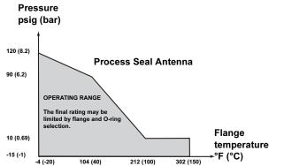
Process temperature and pressure diagram.
