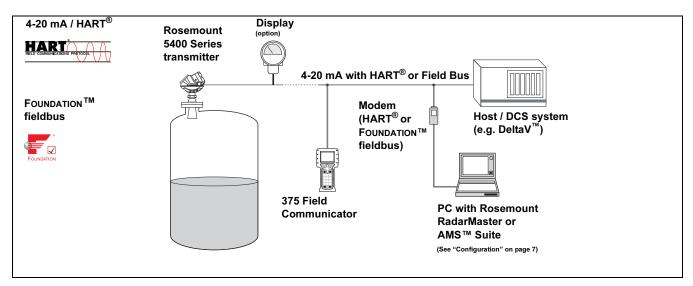
The 5400 Series can be integrated into almost any new or existing plant. Configure it remotely in the control room over the 4-20 mA/Hart® or FOUNDATION™ fieldbus wires. No proprietary connections are needed.
