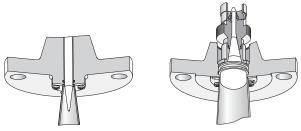
Rosemount 5400 Series transmitters are equipped with an enlarged PTFE tank seal to protect the antenna from contamination and condensation, an especially important feature for high frequency antennas.
