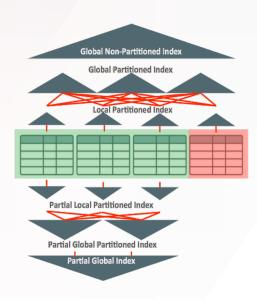
Figure 2: Indexing on partitioned tables
