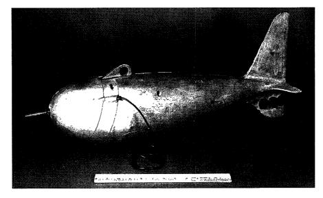
Figure 9. US P-61 point-integrating suspended-sediment sampler.
