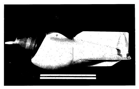
Figure 8. US D-77 suspended-sediment sampler.
