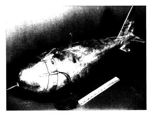
Figure 10. US P-63 point-integrating suspended-sediment sampler.
