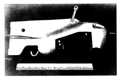
Figure 6. US DH-76 suspended-sediment sampler.
