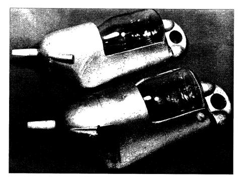
Figure 4. US DH-48 suspended-sediment sampler.
