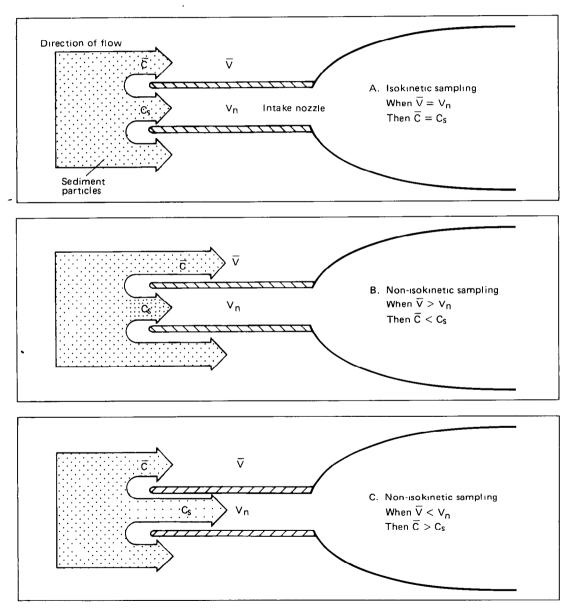
**Figure 11.** Relation between intake velocity and sample concentration for (*A*) isokinetic and (*B*, *C*) non-isokinetic sample collection of particles greater than 0.062 mm. When  $\overline{V}$  = mean stream velocity,  $V_n$  = velocity in the sampler nozzle,  $\overline{C}$  = mean sediment concentration in the stream, and  $C_s$  = sample sediment concentration.
