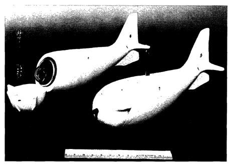
Figure 7. US D-74 suspended-sediment sampler.
