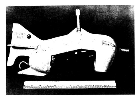
Figure 5. US DH-59 suspended-sediment sampler.
