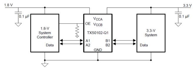
Figure 11. Typical Application Circuit
