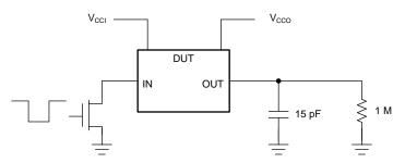
Figure 5. Data Rate, Pulse Duration, Propagation Delay, Output Rise And Fall Time Measurement Using An Open-Drain Driver
