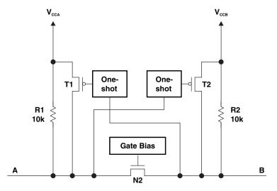
Figure 10. Architecture of a TXS0102 Cell
