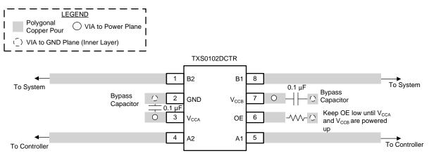
Figure 13. TXS0102 Layout Example
