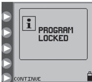
Figure 19. Program Locked screen, which indicates the pump is in LOCK SETTINGS mode.
