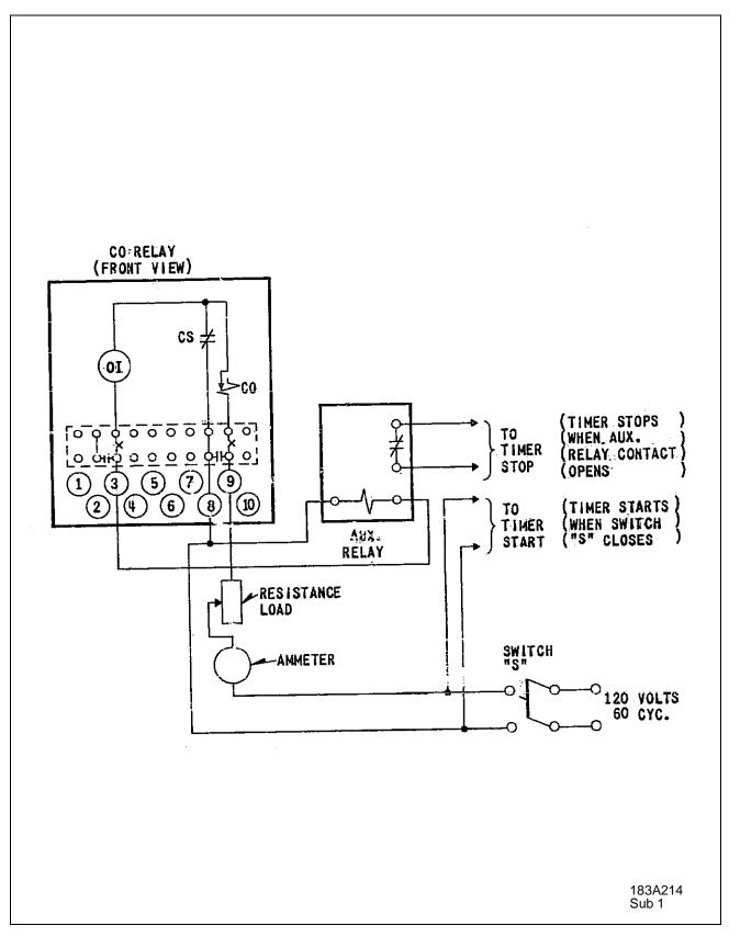
Figure 10: Diagram of Test Connections for the Circuit Opening CO Relay in the Type FT-21 Case
