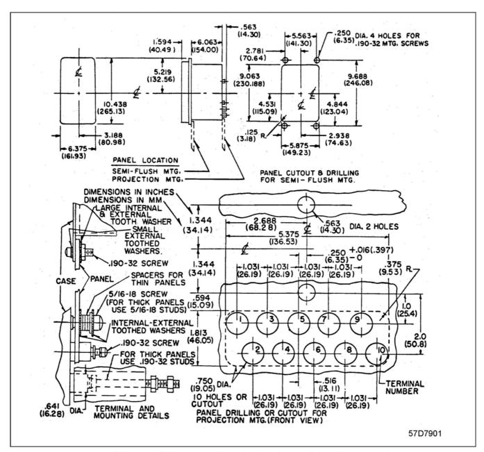
Figure 12: Outline and Drilling Plan for the Circuit Opening CO Relay in the Type FT-21 Case
