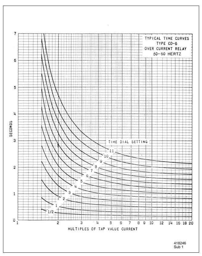
Figure 5: Typical Time Curve of the Type CO-6 Relay
