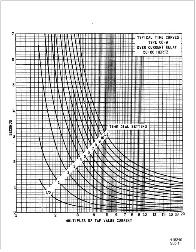
Figure 8: Typical Time Curve of the Type CO-9 Relay
