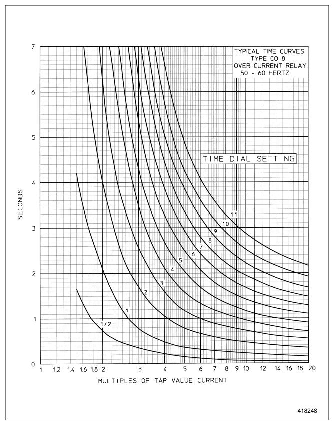
Figure 7: Typical Time Curve of the Type CO-8 Relay
