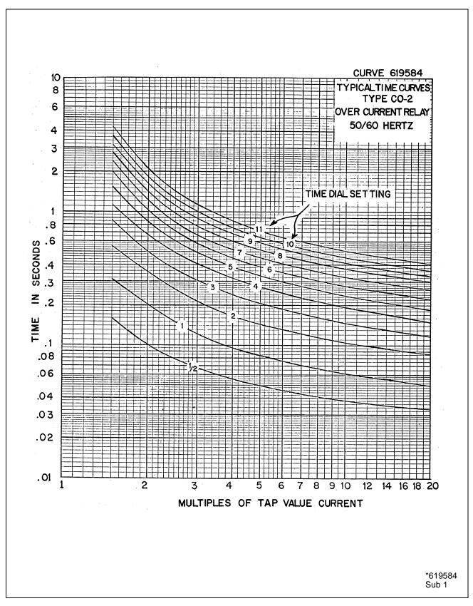
Figure 3: Typical Time Curve of the Type CO-2 Relay
