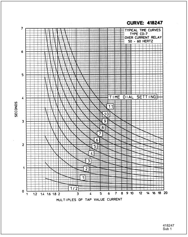
Figure 6: Typical Time Curve of the Type CO-7 Relay
