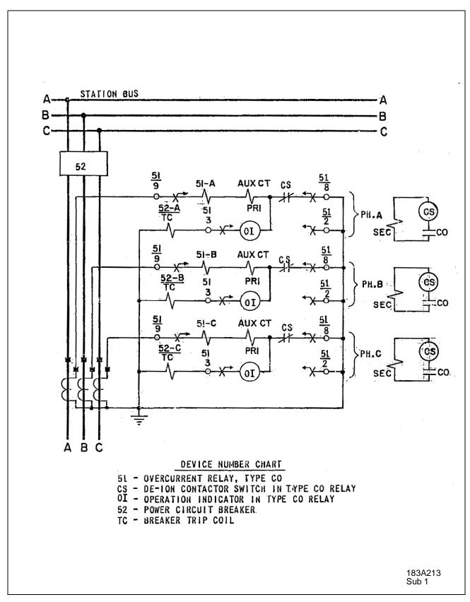
Figure 11: External Schematic of the Circuit Opening Type CO Relay for Phase Overcurrent Protection on a Three Phase System
