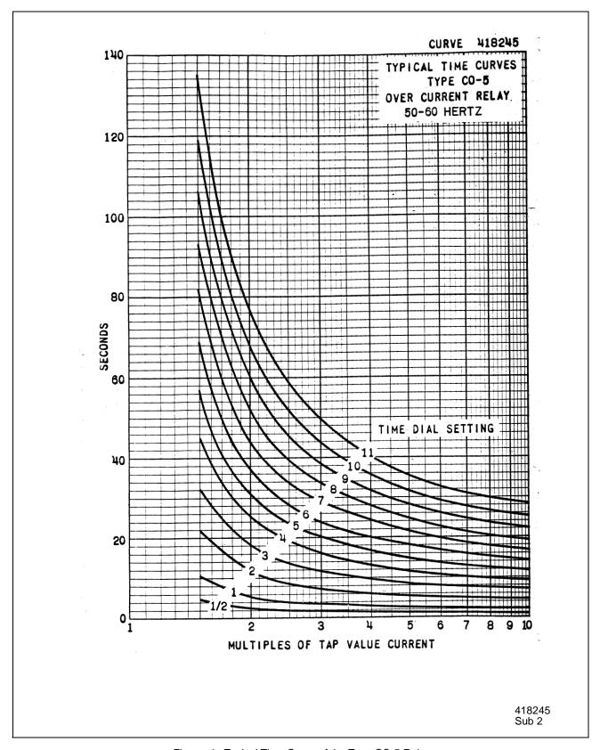
Figure 4: Typical Time Curve of the Type CO-5 Relay
