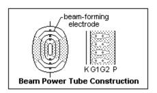
creating a shadow, in which the screen grid was located. This greatly reduced the screen current, and increased the permissible plate current. The space charge of the electron beam served to drive secondary electrons back to the plate without the necessity of a suppressor grid, although in some cases the suppressor may be
