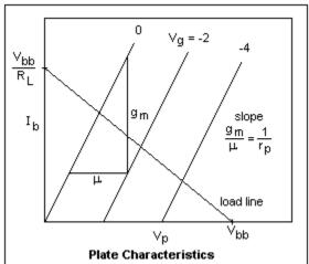
represented by the line labelled  $\mu$ , is the amount the plate voltage must increase to hold the plate current constant; it represents the relative influence of plate and grid on plate current, and is the *amplification factor*. The vertical distance between them
