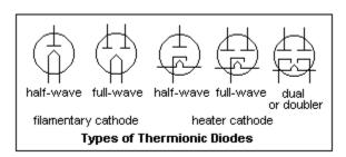
an electron-receiving anode or plate. The arrangments of cathodes and plates in commercial tubes, and what they are called, are shown in the figure. Signal diodes are also often added to a triode or pentode, sharing the same cathode and with one or two plates. Current flows only from plate to cathode, and this unidirectional conduction is the purpose of a diode. Diodes cannot amplify.
