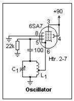
An oscillator using a 6SA7 pentagrid converter is shown at the left. A 6BE6 can be used instead, if you wish. The circuit will not oscillate with an unbypassed resistor in the plate lead, but you can measure the DC plate current with a DMM instead.  $L_1$  is an
