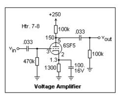
A voltage amplifier using the 6SF5 is shown at the left. This circuit makes quite a contrast in gain with most of the circuits we have seen so far. The gain is about -47, input to output. The plate current is 1.0 mA, making the plate voltage about 150V. The load consists of a 100k plate resistor, and a capacitor-coupled 100k resistor representing the grid resistor
