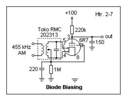
The rectified signal voltage is of the correct polarity to provide grid bias for the amplifier tube in this circuit. Therefore, the grid of the triode can be connected directly to some point on the diode load resistor that provides the proper bias, in place of the volume control potentiometer and coupling capacitor shown above. This arrangement is called *diode bias*, illustrated by the circuit at the left. AVC is essential when diode bias is used, to
