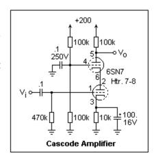
gives both triodes sufficient "headroom" to operate reasonably. This circuit gives an overall gain of a little more than -50, while the gain from the input to the plate of the lower triode is about -3, making the gain of the upper triode +17. There is no advantage whatsoever to returning the capacitor bypassing the upper grid to the input (as shown in Langford-Smith's circuit, Figure 12.51B).
