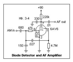
A detector-amplifier circuit is shown at the left. This circuit is fed by a signal generator at AM in, and the audio output is taken from AF out. The amplifier uses grid-leak bias, which effectively clamps the peak of the audio wave at 0 V. The stronger the input signal, the more negative the grid bias, which makes the most of what is there. With an AM input of peak value 0.95 V and modulation amplitude 0.37 V, the peak to peak
