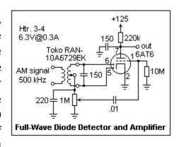
got 26V peak-to-peak at the plate of the 6AT6. The RF ripple was negligible, but there was some 60Hz pickup, not surprising with a high-gain breadboarded circuit out in the
