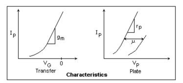
found  $\mu=22$  (at 7 mA plate current),  $g_m=2.9$  mS (at 90V plate voltage), and so  $r_p=7.6$  kO, quite close to the published values. These values are not constant, of course. Verify that  $\mu=g_m r_p$ . Find the cutoff bias for some value of plate voltage. Since this point is not definite, it is usually defined as the voltage at which the plate current drops to some small value, say 10  $\mu$ A.
