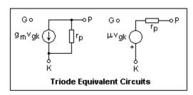
source. It shows the significance of the amplification factor, and is useful for triodes because of the rather small plate resistance. We did not find the Th%eacute; venin source for transistors very useful, and did not introduce a parameter analogous to the amplification factor for this reason.
