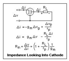
It is most enlightening to consider the circuit as a common-cathode amplifier driving a common-grid amplifier. To estimate the gain of the common-cathode stage, the impedance looking into the cathode of the common-grid stage must be known. The box at the left shows how to do this. A change in voltage? v is applied to the input, and a change in current? i results. The ratio is the input impedance. The circuit shows changes only, so the load resistor is returned to ground, instead
