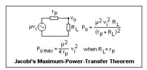
the square of the input voltage on the grid. Maximum power is developed when the load resistance is equal to the plate resistance, other things equal. This is an application of Jacobi's maximum-power-transfer theorem. The power is then given by the square of the input voltage times a factor called the *power sensitivity*,  $\mu^2/4r_p$ .
