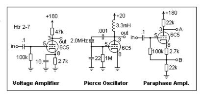
potential 98V, and the gain was -15. The gain was closely predicted by the load of 47k||11k| and the transconductance of 1.8 mS. The plate current was 1.67 mA. As usual, small plate currents are used in voltage amplifiers so that the plate resistor can be as large as possible.
