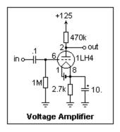
The 1LH4 is a loktal battery triode, which is shown in a voltage amplifier at the left. A similar octal tube is the 1H5-GT, and either will do in this experiment (but the basing is different!). A diode plate is included, connected to pin 4, and using the negative side of the filament as its cathode. The diode is not used in this circuit. The maximum plate voltage is 110V, but this can be exceeded a little in testing. I measured the characteristics for plate voltages of 125V and less, at grid
