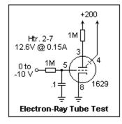
A circuit for testing an electron-ray tube with a triode in the same envelope is shown at the left. The 1629 is recommended, as the cheapest and most widely available electron-ray tube. It operates exactly like the 6E5 and similar tubes, which are expensive and should be left to radio restorers. It is an attractive tube, and the internal construction can be seen clearly. Notice especially the continuation of the triode plate as the ray-control electrode. 200 V is required for
