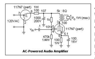
An amplifier using the 117N7 is shown at the left. The 117N7 supplies its own DC power in this circuit, so the circuit is self-contained and makes a convenient line-powered amplifier. The output transformer is a T31 transformer from Antique Electronics (\$12.95), rated at 8W, 5k single-ended to 8&Omega. Its design DC bias current is not given, but is probably
