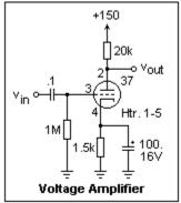
low-mu triodes are not adapted to voltage amplification. The input impedance of 1M means that there is a large power gain in this amplifier.
