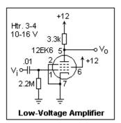
The 12EK6 (also known as 12DZ6 and 12EA6) is a screen-grid pentode for low-voltage use. A voltage amplifier using this tube is shown at the left. This tube was generally used as an IF or RF amplifier, so the load would have been a resonant circuit, not a resistor, giving much higher gain. However, the resistive
