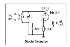
A diode detector, using a standalone diode, is shown at the left. The output is the same amplitude as the modulation on the carrier that is input, very closely, so the detector could not do any better. Often, the diode was included in the first AF amplifier tube, sharing the same cathode, and dual diodes were also available for
