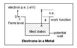
electrons are negatively charged, this means that voltage gets more negative upwards. There are not many more states than electrons, so they fill up the states up to some energy called the Fermi energy at 0 K. At ordinary temperatures, there is little difference, since the thermal energy is small compared to the kinetic energy of the electrons near the Fermi level.
