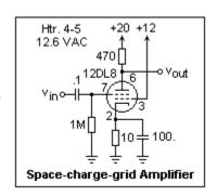
peak-to-peak input, the output is 6.5V, for a gain of -3.25. This is just what is expected from the measured characteristics. The bias current varies with the input voltage (decreasing as the input amplitude increases), and in this case is about 17 mA. The space-charge grid current is 74 mA. These are rather large currents, but the low voltages mean that only modest power is involved. Note that the input impedance is high, set by the 1M grid resistor, and the output resistance is low.
