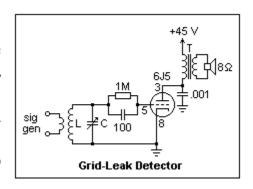
The circuit works, but I was not impressed by its output. Asking for loudspeaker output from a detector is being very optimistic, but I had some hopes. Perhaps a more suitable transformer would give better results.
