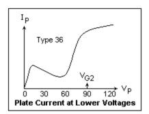
The screen grid should be connected to a constant 90V source, while the plate voltage should be variable from near 0 to about 150 V. Plate voltage and plate current should be measured with DMM's. More details are available below in the section on pentodes. The variable grid voltage supplied by a potentiometer and the C supply should also be measured. I used grid voltages of –
