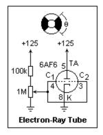
sector. You can easily try this yourself if you want. Some electron-ray tubes (e.g., the 6E5) actually include a triode just for this purpose. The 100k resistor is to protect the
