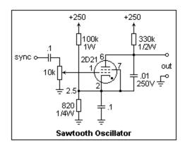
A practical sawtooth oscillator using the 2D21 is shown at the left. The screen grid is connected to the cathode. Control-grid bias is produced by the voltage divider of 100k and 8200. The charging current also flows through the 8200 resistor, so the actual bias is about 2.5V rather that the 2.0V that the divider alone would supply. The 0.1  $\mu$ F capacitor is to hold the cathode potential constant. A larger value would not be wrong. The 330k
