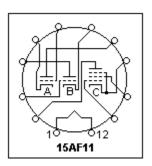
voltages. The transconductance was 5.9 mS at 8 mA, 4.9 mS at 5 mA, and 3.5 at 3 mA. The plate resistance was 60 kO at 10 mA, 130 kO at 7 mA (all by measurement).
