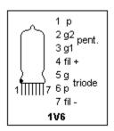
lower plate currents. The two devices can be tested as usual, taking care not to exceed 45V or 1 mA. Note that the pentode and the triode share the same filamentary cathode.
