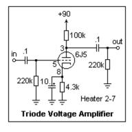
A different resistance–coupled triode voltage amplifier is shown in the diagram on the left. The resistance "seen" by the 0.1  $\mu$ F coupling capacitors is 100k || 220k or 68.8k. The corner frequency of this RC filter is 1/2pRC = 23 Hz, sufficiently low for an audio amplifier. The corner frequency of the cathode bypass is 48 Hz. The predicted gain is roughly  $g_m = 3.0$  mS times 7.7k||100k||220k = 6.9k, or -21. It drops to about -6.9k/4.6k = -1.5 if the cathode is not
