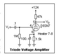
the vacuum tube over the transistor. The cathode resistor of 1.5k sets the quiescent operating point roughly halfway between 0 and 124V, allowing the greatest possible
