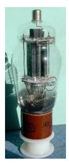
within its amateur (ICAS) or commercial (CCS) ratings. If a plate gets hotter than when it was outgassed at the evacuation of the tube, it may emit gases and ruin the tube.
