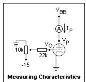
A circuit for measuring triode characteristics is shown at the left. The 22k resistor is merely to protect the potentiometer, and is not essential. A large value, such as 1M, could be used
