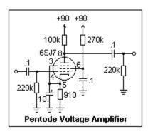
A pentode voltage amplifier using a 6SJ7 is shown at the left. The AC gain of this amplifier is close to  $g_m=1.6$  mS times 68.8k, or -110. It won't be quite this high with a 90V B+, but will still give a lot more gain than the triode amplifier. My 6SJ7 gave a gain of -60 at  $V_{bb}=90$  V, and  $V_p$  was 27.2 V, showing that the plate current, 0.63 mA, should be reduced a little to raise the plate to about 45 V. The 6SJ7 tested was very close to specifications, despite
