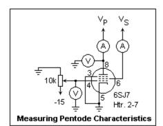
The circuit for measuring pentode characteristics is shown at the left. The tube used as the example is the 6SJ7, but any sharp-cutoff pentode will do, such as the miniature 6AU6. It makes things very easy if you have four DMM's for the various measurements. The screen supply can be fixed-voltage. I used 105 V from a VR tube at first, later the all-in-one supply described
