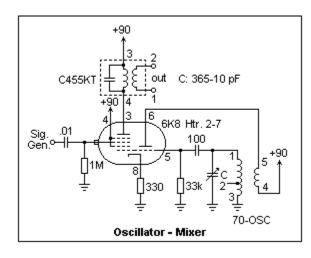
An alternative to the pentagrid converter is the triode-hexode converter. In this tube, the oscillator plate is separate, while the oscillator and mixer share the same control grid. The RF signal to be converted is applied to grid 3 of the hexode, grids 2 and 4 acting as a screen. This very well isolates the oscillator from the RF. The 6K8 is a good example of a triode-hexode converter. The circuit at the left can be used to study its action. The RF input is usually an antenna
