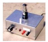
The voltage regulator requires a certain minimum current (about 5 mA) to function properly. If you are only drawing a few milliamperes from the supply, connect a 12k bleeder resistor across the output. Otherwise, the regulator will not adjust down to the lower voltages. Or, 220O and 10k fixed resistors, and a 15k pot, could be used at the voltage regulator, which would
