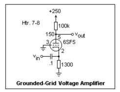
The circuit at the left shows that the signal can be input to the cathode instead of to the grid, in what is called a *grounded-grid*, or common-grid, amplifier. If you test this circuit, you will find that the gain is +50. However, the input impedance is now quite low, about 3820, so power is required to drive it. Also, note that the input coupling capacitor is  $0.1 \mu F$ , and even so the gain drops at low frequencies because of
