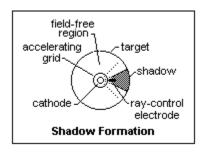
If the ray-control electrode is at a lower potential than the target, it deflects the electrons away from itself, symmetrically on either side, so that no electrons move in a sector centered on the electrode. This is shown in the figure at the left. The more negative the ray-control electrode, the wider is the sector. When it is at the target potential, there is no dark sector. It is easy to see why the
