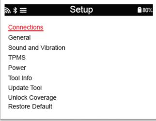
**Connections** Connect to a Bluetooth OBDII Module, TPMS Desktop, and WiFi.
