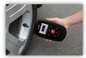
(Note: with Ford Banded sensors the tool should be held 180°/opposite from the stem's position)
