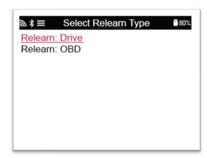
To find out which relearn type is available for a vehicle, just turn on the tool and select Relearn. Or refer to the current coverage list at <a href="https://www.bartecautoid.com">www.bartecautoid.com</a> > Downloads.
