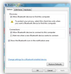
Right click on the Bluetooth dongle icon and click on Bluetooth settings. Tick the boxes as seen on the Options tab above. Press OK when finished. Start the TPMS Desktop application and go to Settings. Open the Bluetooth section: the PC/Laptop should be **connectable** and **discoverable** for the TECH600.
