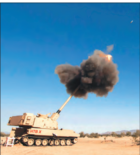
YPG conducts developmental testing of multiple facets of the Extended Range Cannon Artillery project, from artillery shells to the longer cannon tube and larger firing chamber the improved howitzer will need to accommodate them. YPG’s ammunition plant has been instrumental in building multiple experimental formulations, shapes, and configurations for new propelling charges to accommodate the improved projectiles. (US Army photo)
