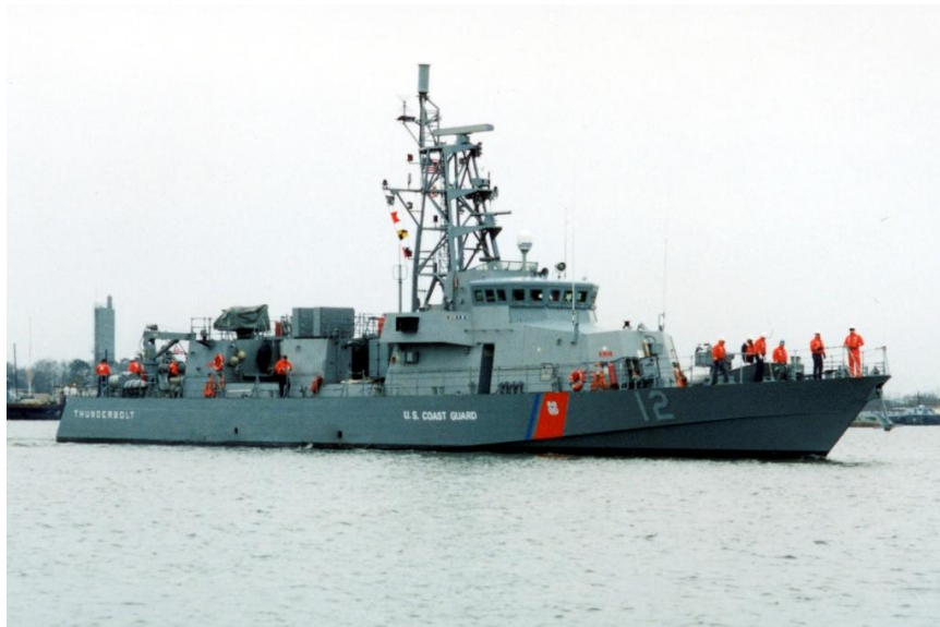
WPC-12 Thunderbolt - circa Mar1998 - being evaluated - note no stern ramp, still 170' long (CG Photo)
