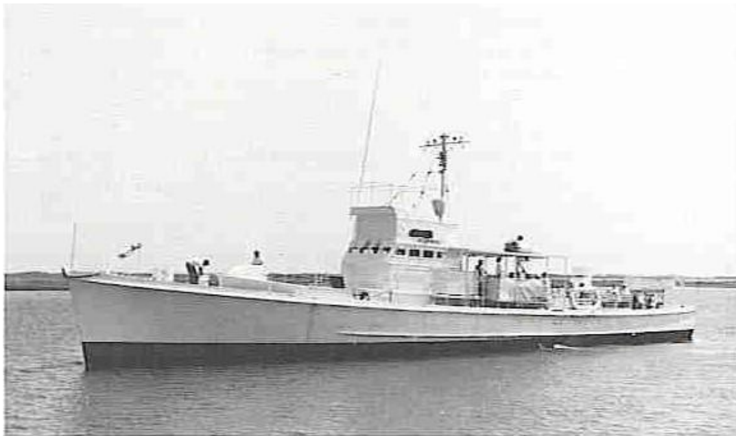
Cutter Air Lapwing on 10 Aug 50. Very few of these 110-foot submarine chasers saw active service in the Coast Guard, primarily due to a severe shortage of personnel.
