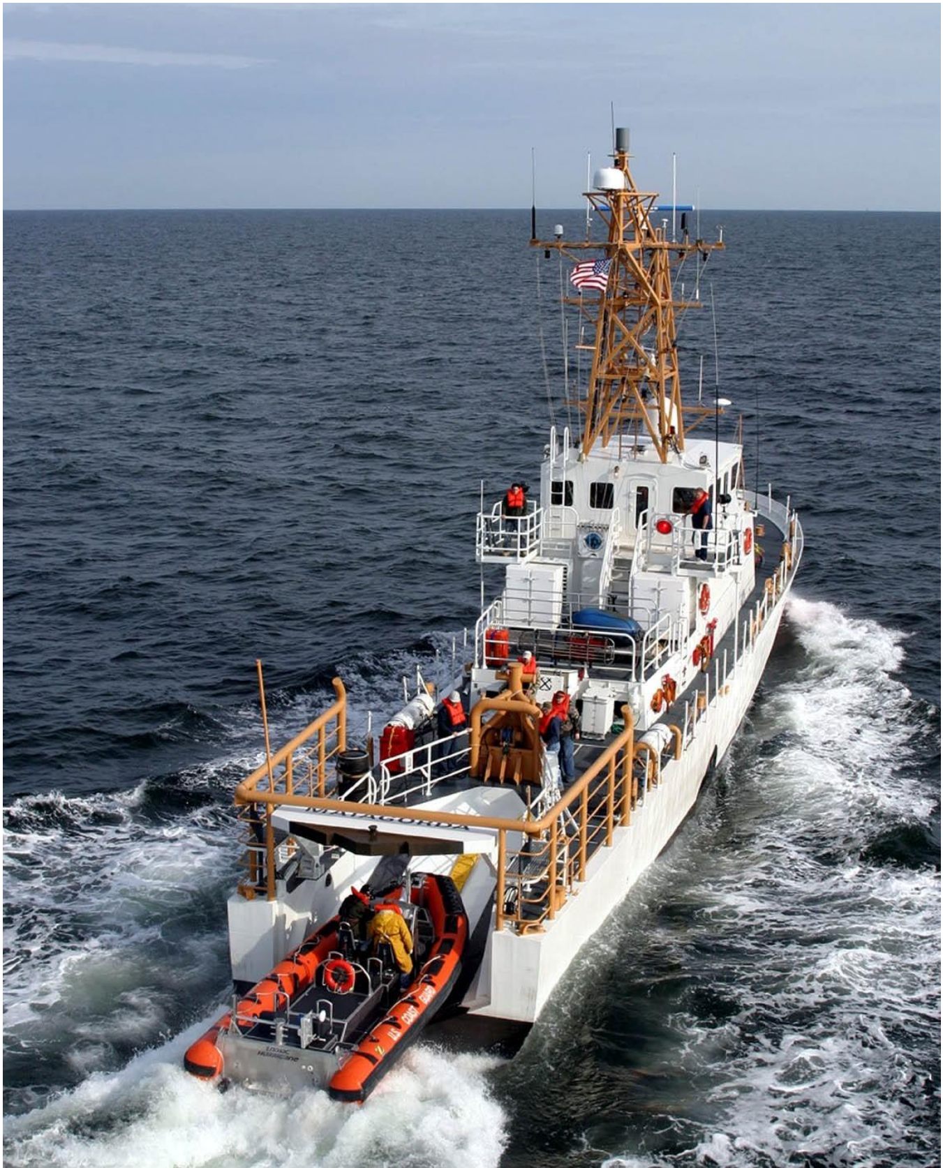
A good look at Matagorda's boat handling system while on trails in 2004. (CG Photo)
